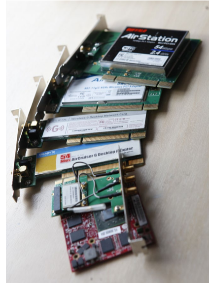
A selection of expansion cards. In the foreground, a laptop graphics card (HD3650) and a desktop adapter for the PCI-E-bus found on laptops; Wi-Fi adapters in the background.
